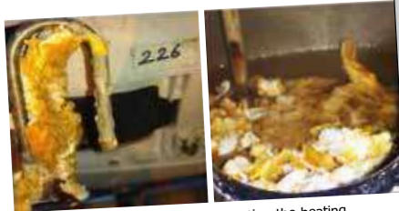
Pictures 2 & 3. Scale previously coating the heating element and reservoir sump. (Picture taken from one of the rooms at IBMA hotel)
