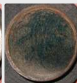
Biofilm in a piping system
