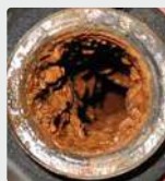
Biofilm in a piping system
