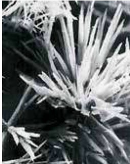
Picture 9: Lime protective layer
