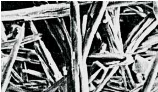
Picture 11: Lime dust deposits
