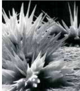
Picture 10: phosphate protective layer
