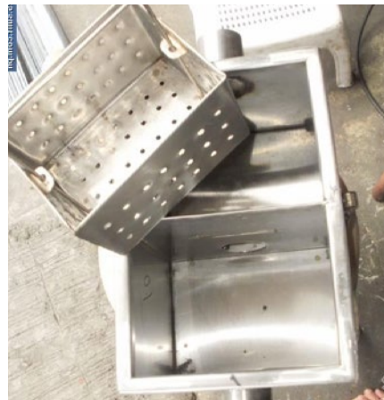
Grease traps have reduced odors and more consistent, less cluttering grease.
