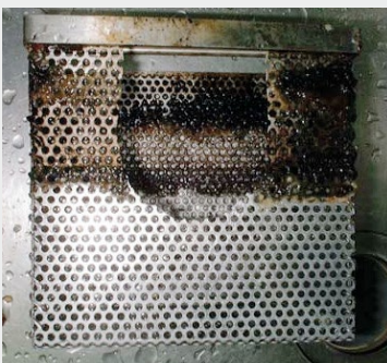
The basket after being washed by hosing. The portions usually being contacted with the treated water are cleaned easily with a water flow from the tap.
