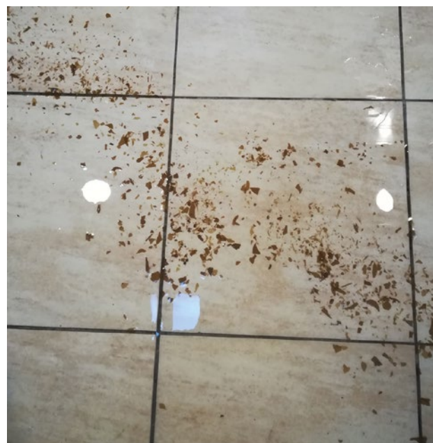
The scale scrap came out of the steamer in the Chinese kitchen.
