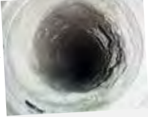
2 weeks after Vulcan was installed, limescale had been softer and fallen out.
