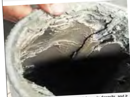
Without Vulcan, the filter was quickly stuck by scale deposits, and it had to be changed every 48 hours.
