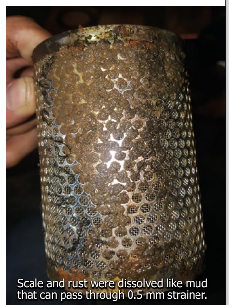
After installing Vulcan S25 for 2 months, scale and rust have been softer and muddy.
