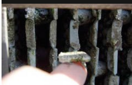
Silica could not be removed by the high pressure water gun, but can be peeled off with a nail.
