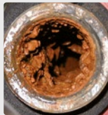
Biofilm in a piping system
