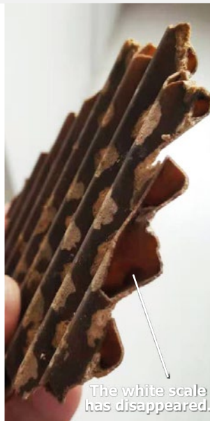
We stopped using any additional chemicals to treat the water. After installing Vulcan S250 for 4 months, the effect was very clear. Although there were still substances in the plate heat exchanger, they had been softened and could be easily removed by hands. There are no more white scales, only yellow-brown impurities left.
