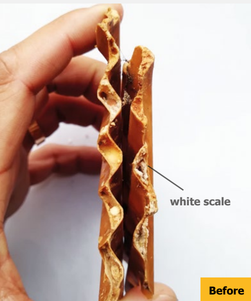
Without Vulcan S250, the plate heat exchanger was scaled badly, and it was almost blocked every month, must be cleaned manually. The scale was hard, could not be removed by hands.
